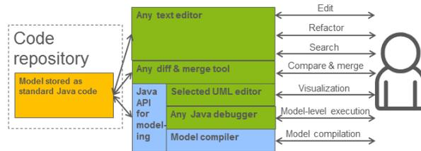
**Fig. 2.** Using an embedded language for executable modeling
