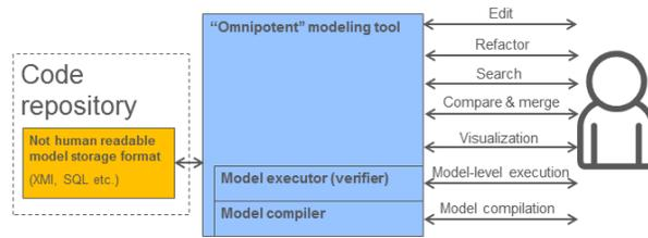
**Fig. 1.** Using an "omnipotent" modeling framework
